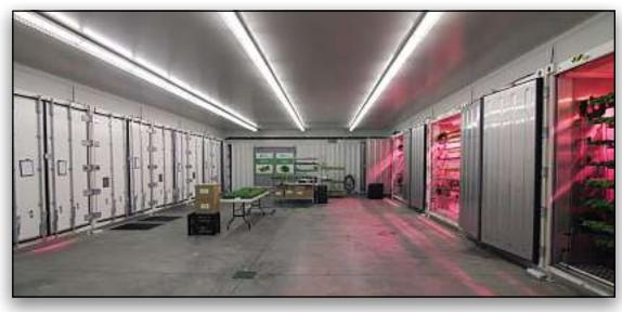
The rotating shelving brings all plants to the front of the growing chamber regularly, eliminating the need for aisle access to reach the plants. (IMAGES COURTESY CUBICFARMS)
